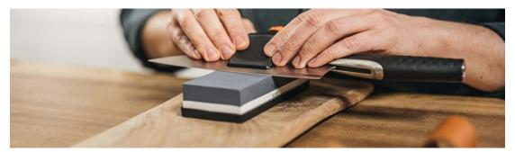
Most modern knives and blades are sharpened by a few passes through an electric sharpener but true experts still prefer to use a whetstone. Made up of rock and grit and wet with water, the whetstone is designed to provide friction that hones the edge of a blade. With a whetstone, you decide how fine the grit is, how narrow the angle, how hard the pressure to determine if the knife is as sharp as it can possibly be. With a whetstone, the outcome is all up to you.
